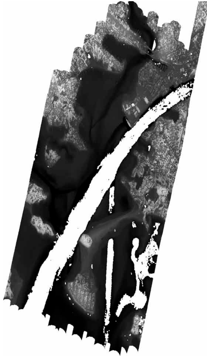
Figure 16. Elevation/depth at Buttermilk Bay Entrance Channel as a result of preliminary processing in DPS for lidar grid generation. Note that the navigation channel running through the middle section of the image is missing data values because the depths are too great to be detected. Lighter shades represent land, while darker shades represent water, or greater depth values.
