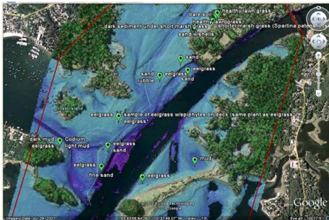
Figure 18. Screenshot of Buttermilk Bay Entrance Channel Google Earth KMZ. The green place markers are sites where spectra were collected using the Divespec underwater spectrometer. The red line is the survey area boundary.
