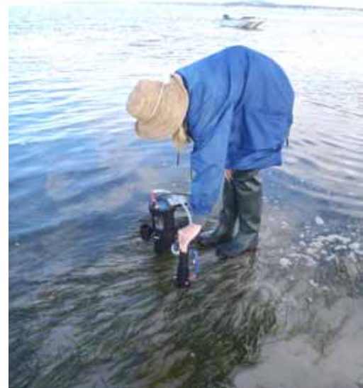
Figure 10. Operation of the DiveSpec in the shallow-water environment measuring SAV reflectance.
